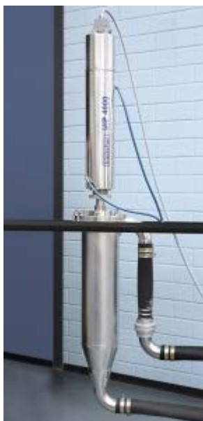
Powerful ultrasonicator UIP4000 for large volume streams
